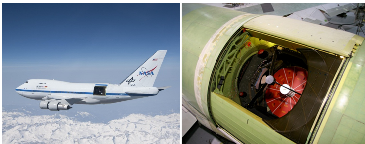
Figure 2. (left) SOFIA is an airborne observatory located in a Boeing 747 aircraft. (right) The 2.5-meter diameter reflecting telescope views the sky during flight through a door built in the fuselage of the aircraft.
