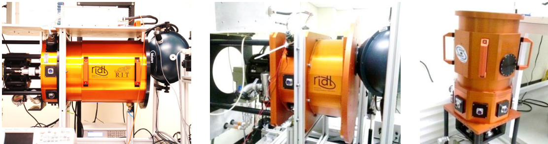
Figure 44. Detectors are evaluated in three custom dewar test systems.
