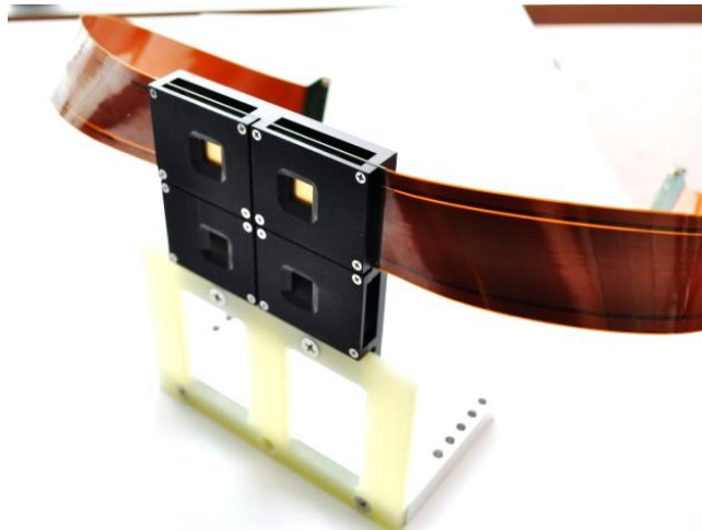
Figure 15. The detectors are mounted to a raft and mount for cooling to cryogenic temperatures. Four detectors are included in this mosaic mount.
