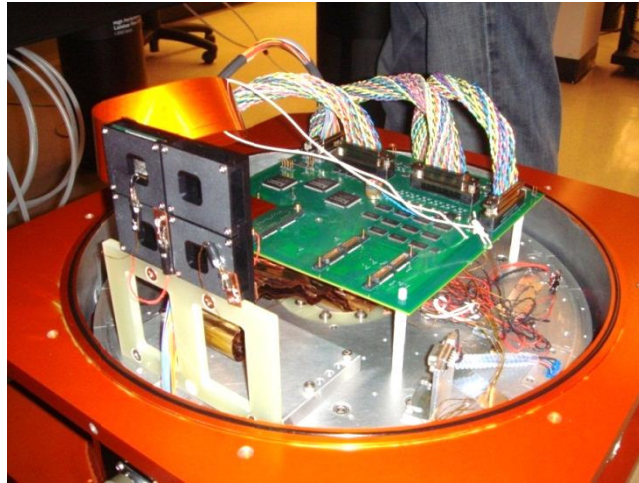
Figure 17. Shown here is the top view of fully integrated detector electronics system inside the dewar. The detector is mounted on the raft and connected to the cold fanout board.
